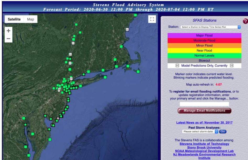
Figure 3. The Stevens Flood Advisory System (SFAS). SFAS is an ensemble-based probabilistic flood forecasting system providing total water level forecasts for coastal and estuarine waterways spanning the U.S. Mid-Atlantic and Northeast.
