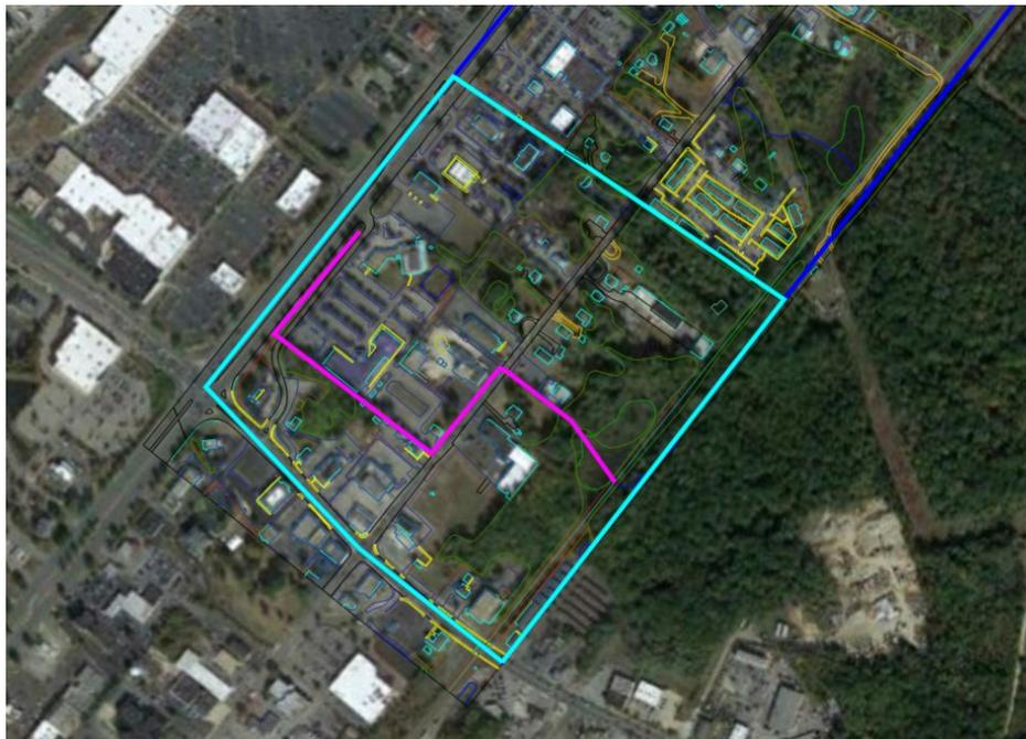
Figure 6. Southern portion of WURC. 65-acre modeled area is highlighted in light blue. Assumed runoff flow path is shown in pink.
