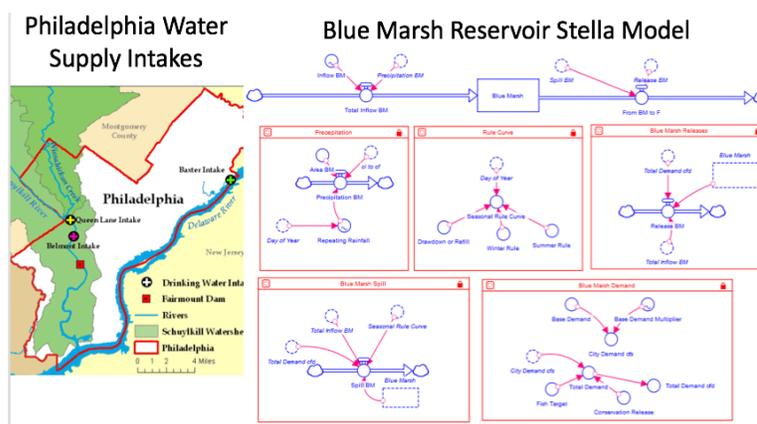
Figure 2. Streamflow model of the Schuylkill River and Delaware River.
