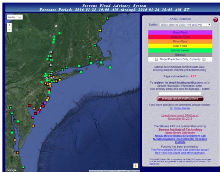
Figure 5. The Stevens Flood Advisory System (SFAS). SFAS is an ensemble-based probabilistic flood forecasting system providing total water level forecasts for coastal and estuarine waterways spanning the U.S. Mid-Atlantic and Northeast.
